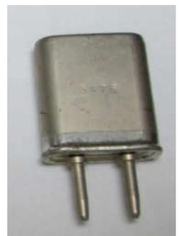
Two FT241 or FT243 crystals will fit into an Octal valve socket.
