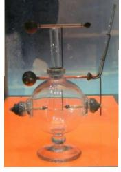
a spherical capacitor, consisting of a smaller sphere inside a larger one, with a gap between them that could be filled with air or anything else. Careful experiments with this device showed that electricity was not a weightless fluid and enabled him to measure the dialectic constant or permittivity of a substance.
