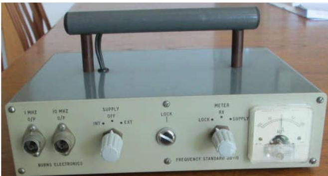
The internal low drop out regulator and battery charger are working well and the unit may be operated from the internal battery with or without float charging or an external 12v DC supply.
