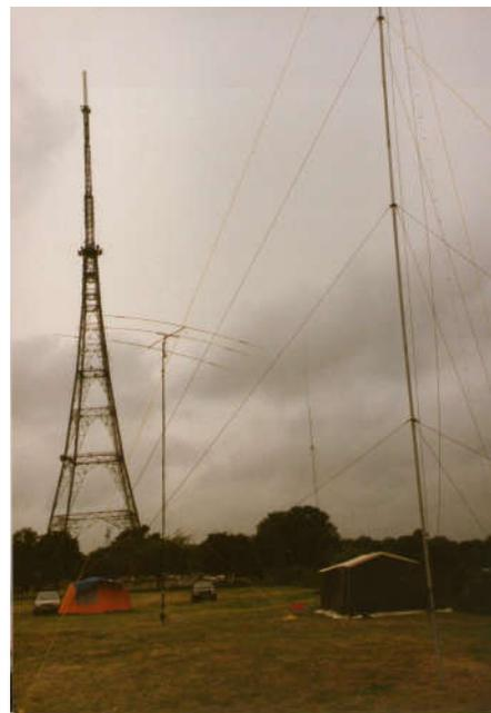
Before we had the beam, an end fed 264ft long Zepp was used, pointed at North
