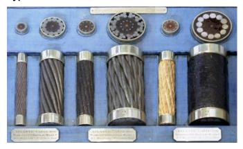
The cable on the extreme left has a diameter of 1.125 inches
