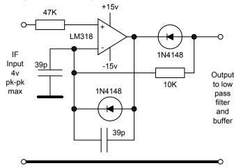
In the interests of simplicity supply rail decoupling has been omitted. Circuit provided by WA1QIX
