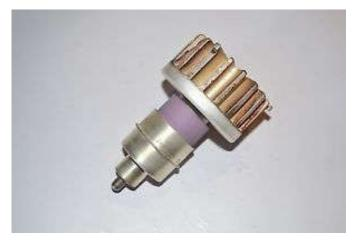
2000 volt supply which is similar to the 4CX250B. However, the grounded grid power gain is only 12-13dB so some 20 - 30 watts of drive is required.
