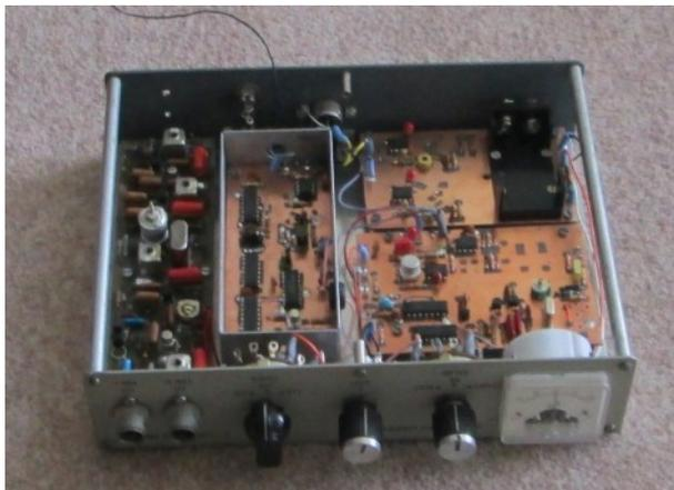
The receiver and crystal filter is on the left, next to the right is the screened enclosure containing the divider system and phase detector. The 10MHz VCXO, divider and loop filter is immediately behind the meter and the unit at the back right is the power supply module containing the charger and battery holder.
