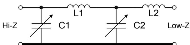
The Pi-L network is, as the name suggests, a combination of a Pi and an L network with the value of C2 being the sum of the capacitors from the Pi and L networks. The output impedance of the Pi network and the input impedance of the L network must be the same value which is usually chosen to be the geometric mean of the anode load impedance (3500ohms) and the output impedance (50 ohms) so in this case about 420 ohms.
