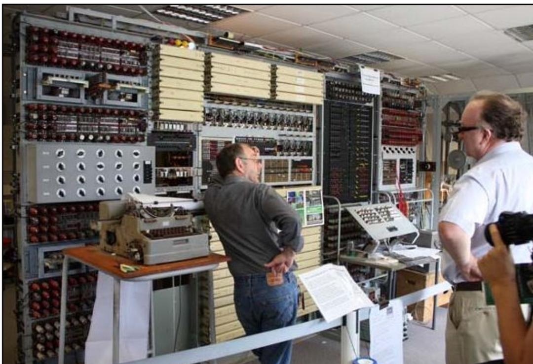
Rebuild of a 1944 Colossus Mk2 computer being used to find the 12 wheel settings on a German Lorenz cipher machine which was used to encipher an intercepted German teleprinter message. The message had been punched onto paper tape (see previous page) and loaded as an endless loop on the right hand end of Colossus (in this photo, it is behind the man in the pale blue shirt who stood in front and wouldn't get out of my way!)
