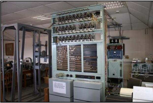
Rebuild of "Tunny" machine used to decipher teleprinter messages
