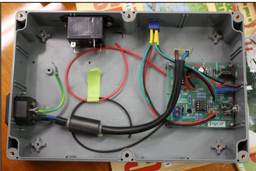
A "Silicon Chip" design also featured in the lead-acid battery condition tester built by Bill Cousins. This unit loads the battery under test to draw an appropriately high current briefly and measures the terminal voltage while under load, registering the result on a series of LED's. This provides an indication of battery condition on a good/fair/poor/fail basis.
