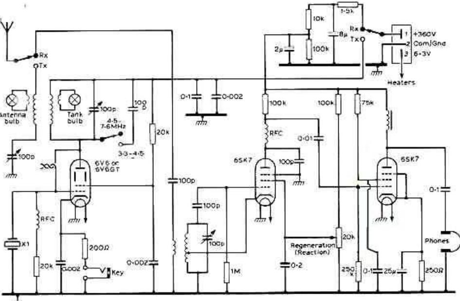
Finally a fairly conventional A.F. amplifier using a second 6SK7 valve amplified the audio signal for application to a pair of headphones.
