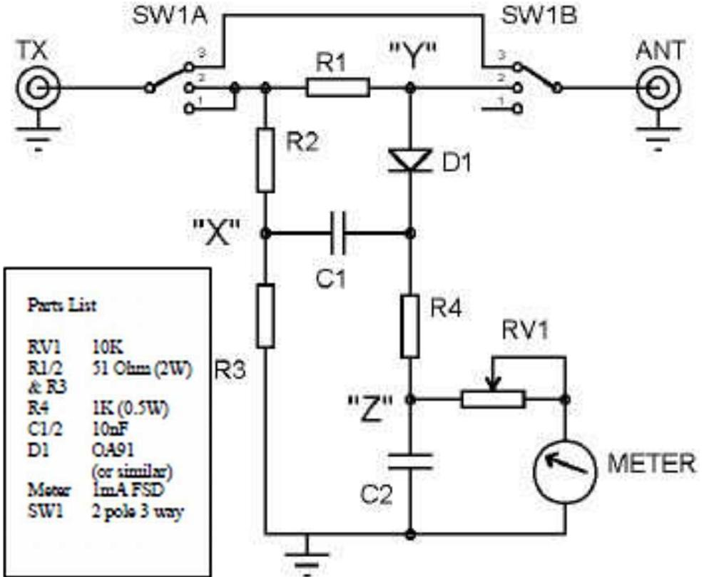
The aspect that catches most out is the fact that the meter is connected to ground and not to point X. The reason for this is that as far as the meter is concerned it is only interested in indicating the DC component. If it is connected to earth, VR1 has only to be reduced in value by the value of R3 to give the same reading. In practice, as VR1 is going to be in the order of kilo ohms compared to the 51 ohms of R3, this error can be ignored.
